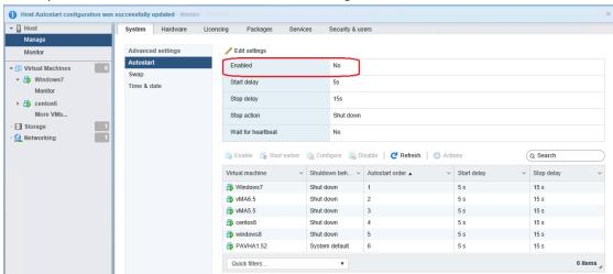
Please choose "Shutdown VMs" checkbox, so Software will shut down the VMs firstly then shut down the host.
