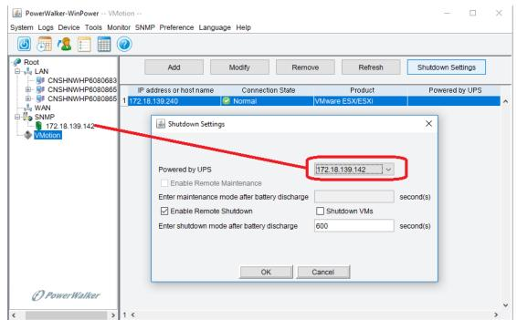
Choose the checkbox "Enable Remote Shutdown", set the UPS discharge timer for ESX/ESXi shutdown
